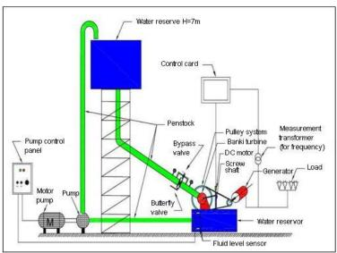
Fig. 1 general appearance of the system which works in closed loop.
